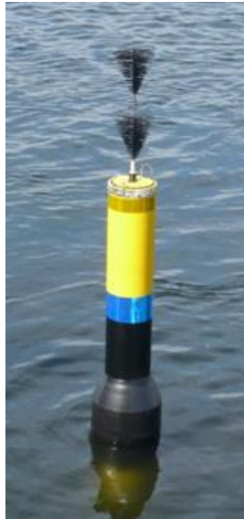
Figure 15 South Cardinal, Comprehensive Code, double blue band and single yellow band (DMA)
