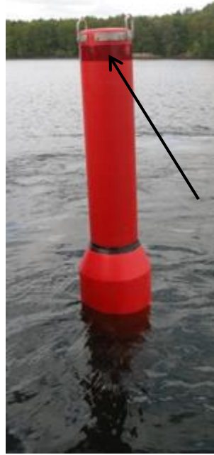
Figure 31 Red lateral spar buoy with horizontal retroreflective band on full circumference of the buoy
