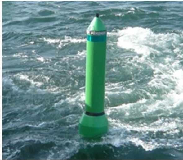
Figure 14 Spar buoy with green retroreflective band (DMA)
