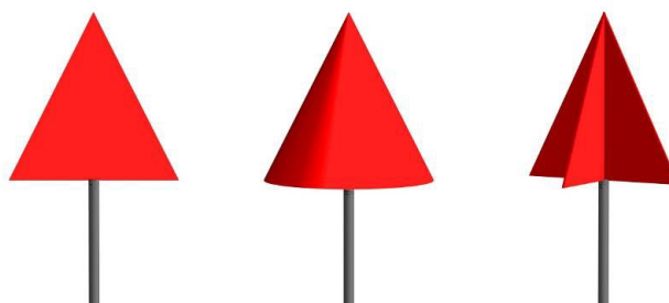
Figure 17 Direct illumination of a daymark (flat, cone, crossed plates)
