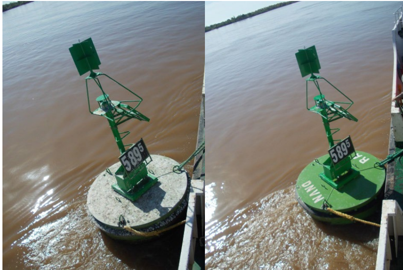
Figure 11 Coated buoy before and after pressure washing
