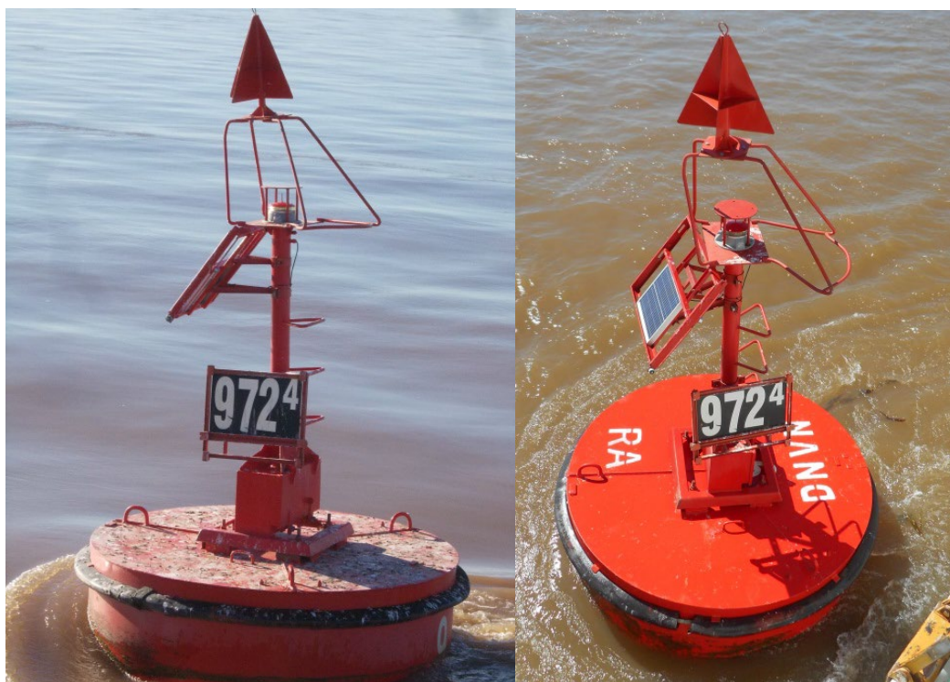
Figure 9 Buoy with modified paint system
