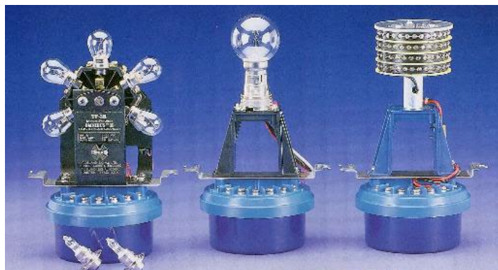
Figure 20 Lensed LED (right) cluster - generally not suitable as a light source in traditional lens systems
