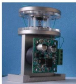
Two side-emitting LED for buoy (the biDE, Source: CETMEF)
