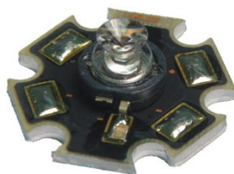
Figure 11 Example of LED heat dissipation package: side-emitting Luxeon emitter
