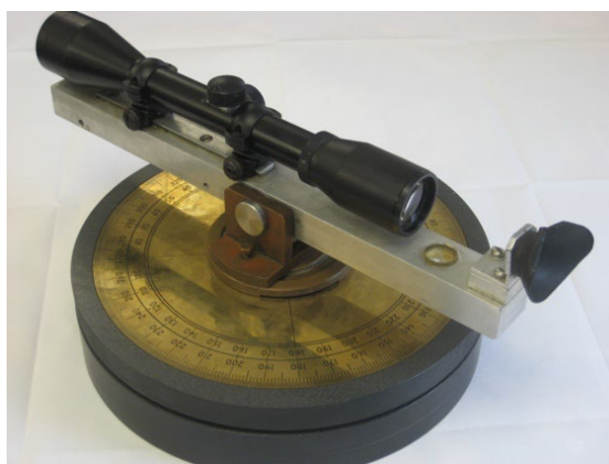
Figure 56 Simple mechanical theodolite
