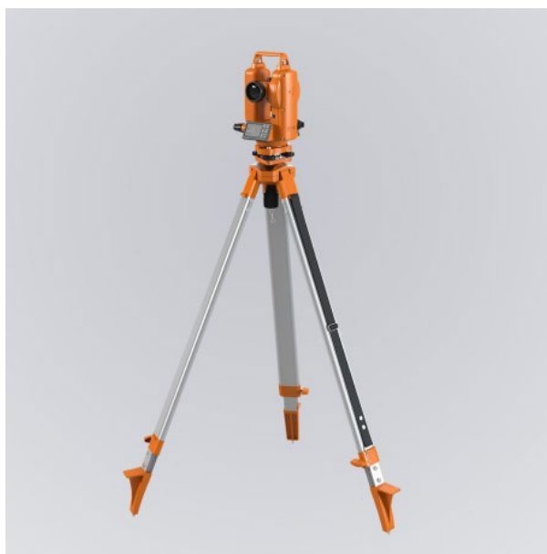
Figure 57 Modern theodolite mounted on a tripod
