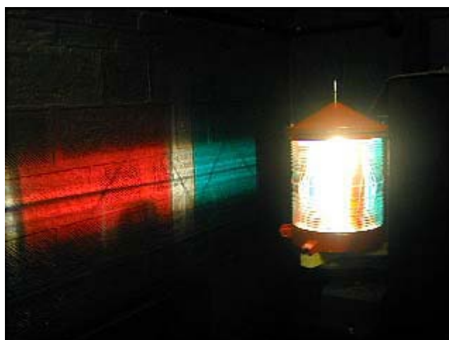
Figure 4 Single light source sector light with drum lens
