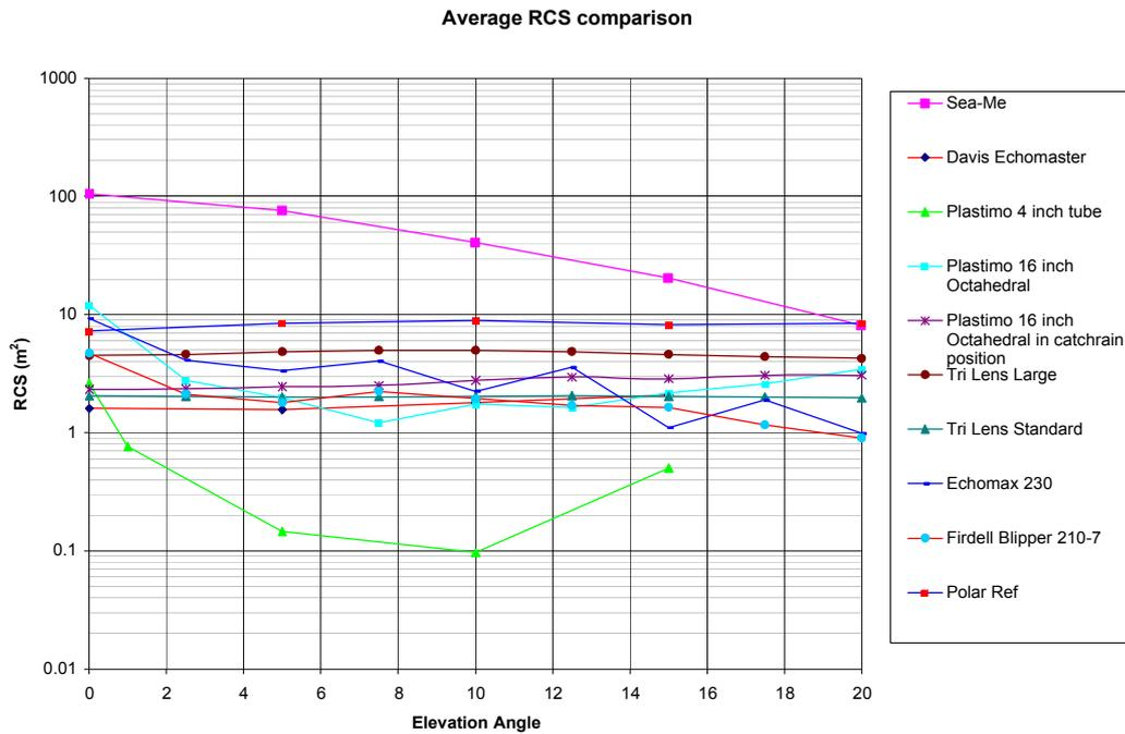
Figure 23 Comparison of each of the radar reflector's average RCS.
