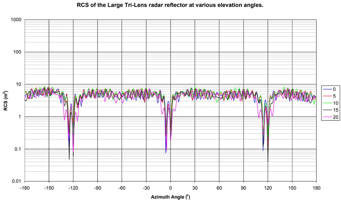
Figure 16 RCS of the Large Tri-Lens radar reflector.
