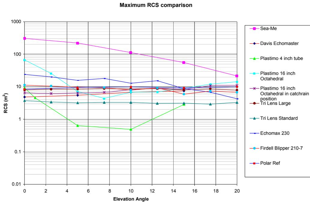
Figure 22 Comparison of each of the radar reflector's maximum RCS level.
