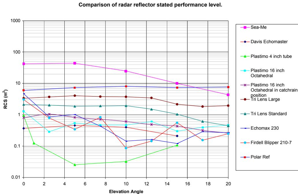
Figure 24 Comparison of each of the radar reflector's stated performance level.
