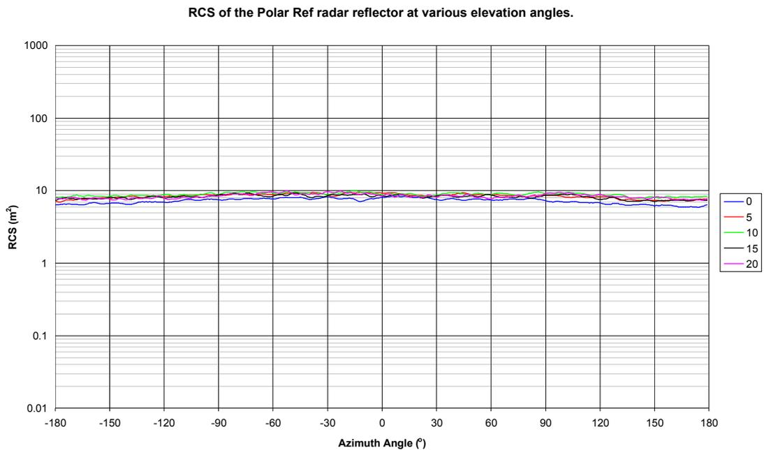
Figure 21 RCS of the POLARef radar reflector.
