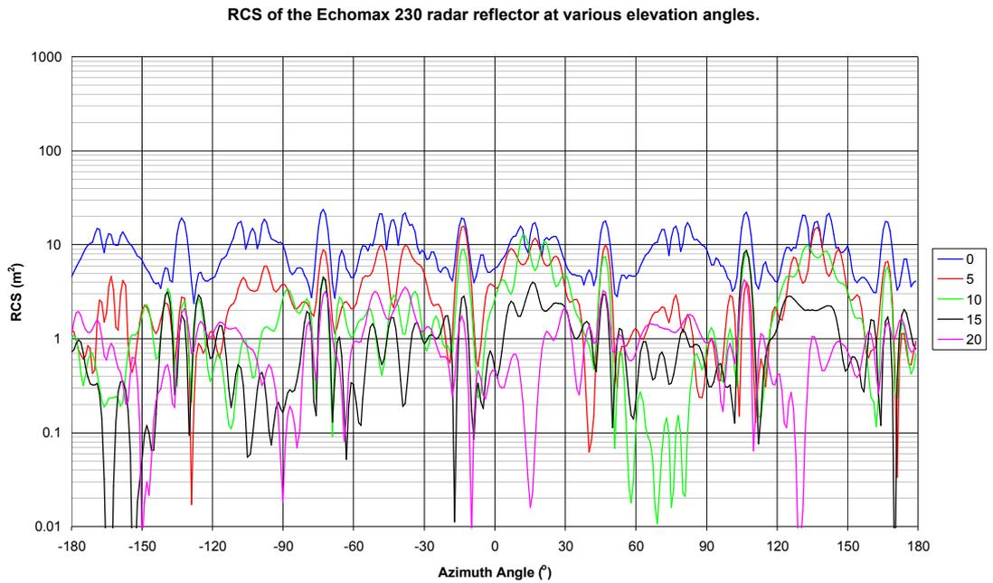
Figure 18 RCS of the Echomax 230 radar reflector.
