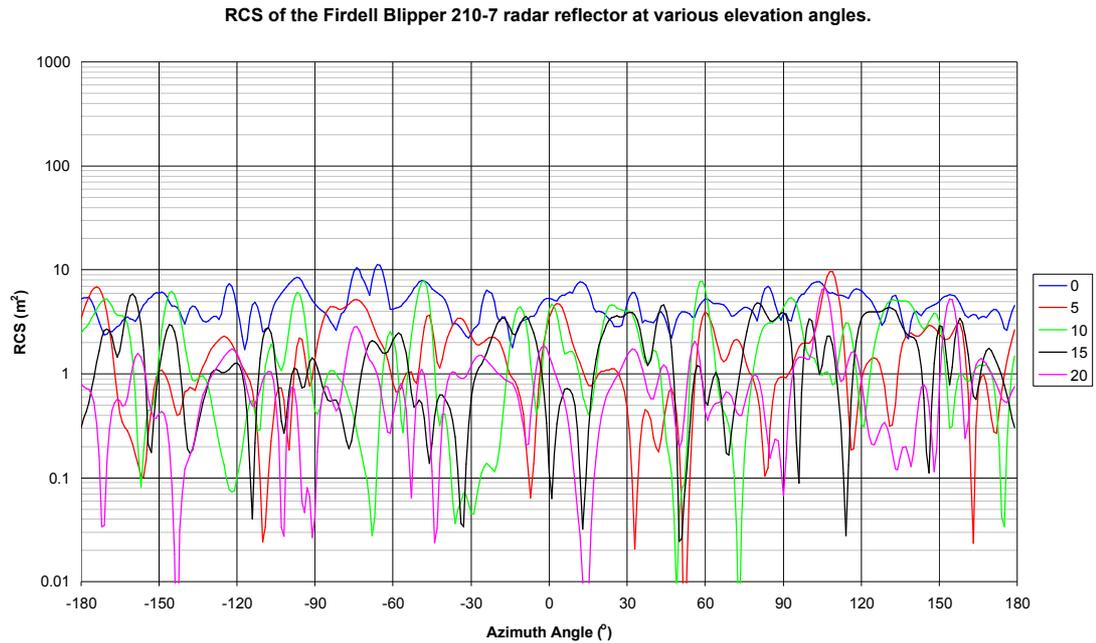
Figure 19 RCS of the Firdell Blipper 210-7 radar reflector.
