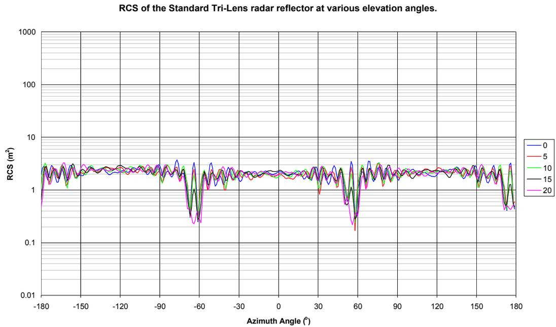
Figure 17 RCS of the Standard Tri-Lens radar reflector.
