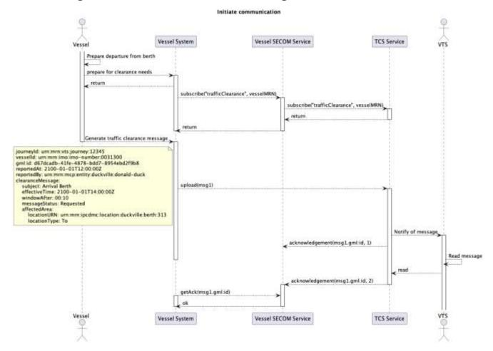
As seen in the diagram, the first step is to use the upload interface of the service to send the initial traffic clearance message to VTS. Once the traffic clearance service has forwarded the message to the VTS system and gets confirmation that the message has been opened and SECOM acknowledgment must be sent. For this to work, the vessel must have subscribed to traffic clearance messages for the vessel so that the service has an endpoint to which to send the acknowledgment message.
