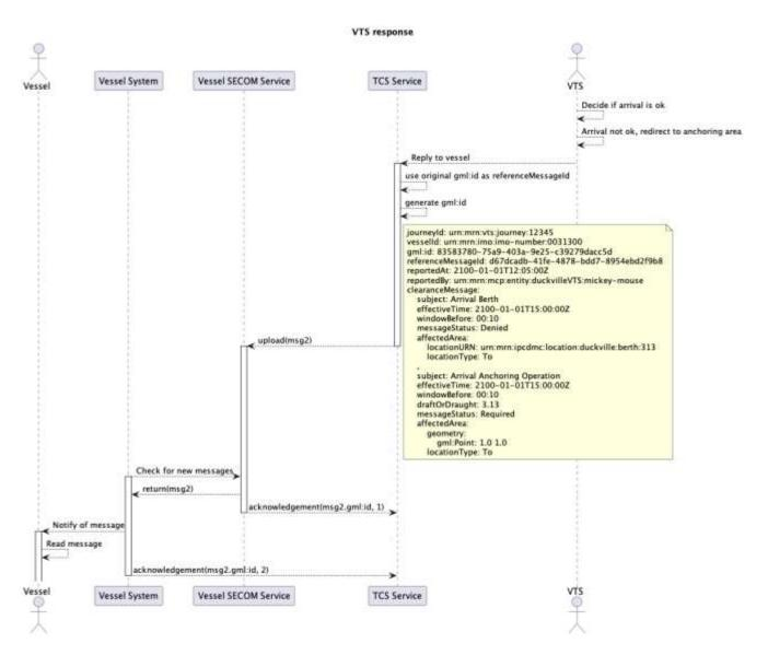
As is the case in the initial upload an acknowledgement must be requested once the message from VTS has been read on the vessel. Not just when it has been technically delivered.
