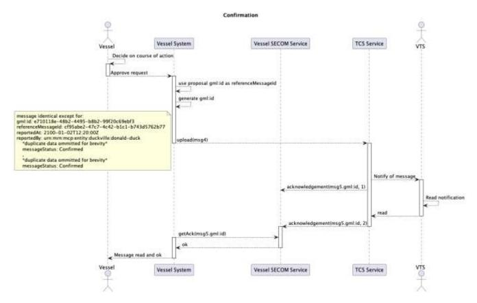
If the messageStatus of the received message is one that does not require an action (i.e. Confirmed, Denied, Cancelled) a response is no longer needed and the read acknowledgment is sufficient to signal that the message has been read and accepted. It is important to note that if the message was sent with a messageStatus of Denied, unless the vessel changes route a new clearance should be requested.
