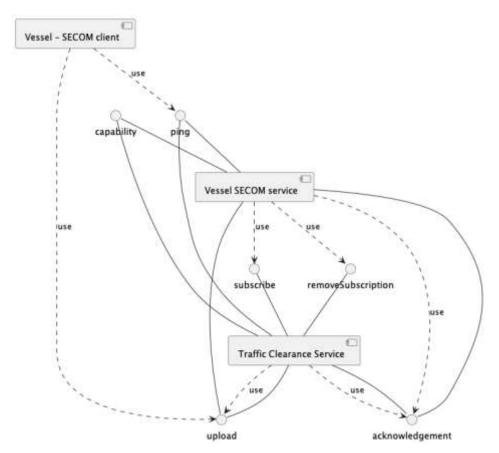
The following diagram illustrates the most extreme use case of the communication between the service and client and illustrates the need for all the interfaces. This example assumes that service endpoint is already known through prior configuration or service discovery from a service registry. Note, the data is not XML in this example and parameters only contain the payload required to describe the business logic.
