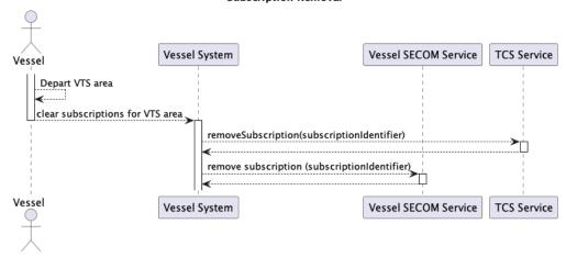
Once the vessel is leaving the area of the VTS the subscription to traffic clearance messages should be removed by calling the removeSubscription interface of the traffic clearance service.
