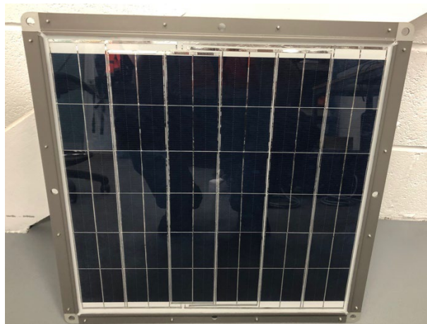
Figure 4 An example of a module with 6 parallel sections
