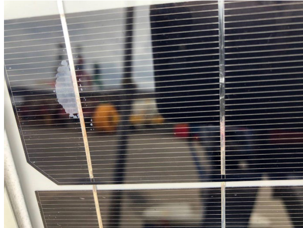
Figure 39 Delamination on a new solar module
