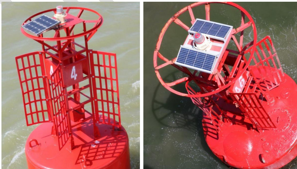
Figure 24 Wind impact to solar modules on buoys
