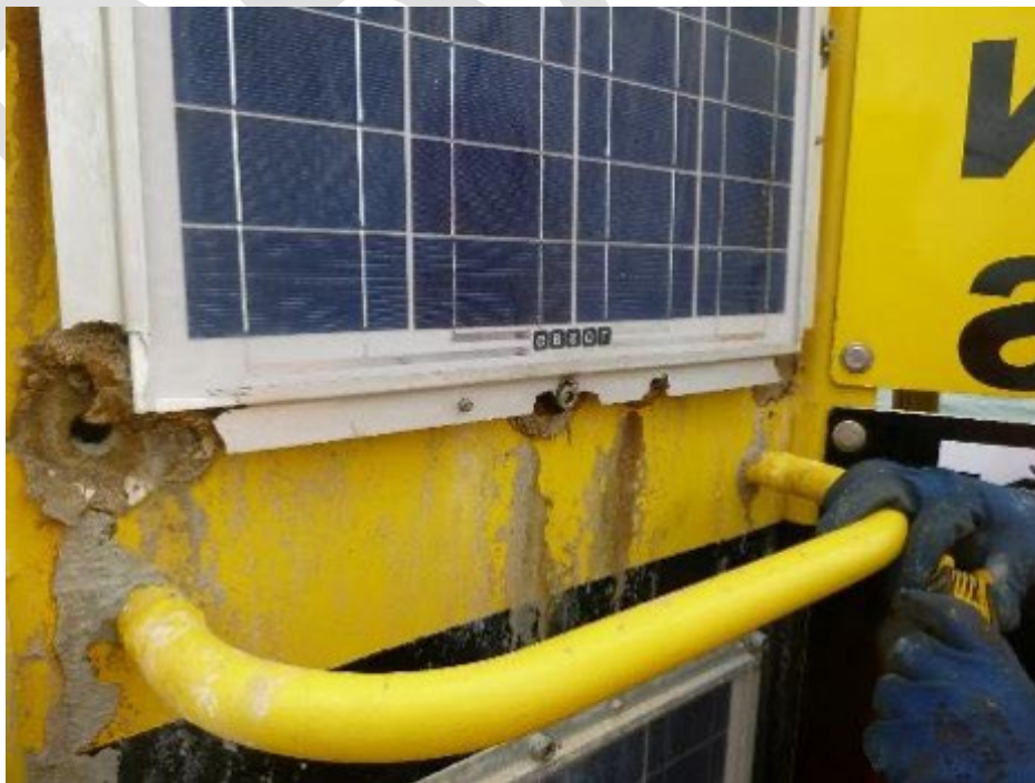
Figure 36 Impact of leakage current
