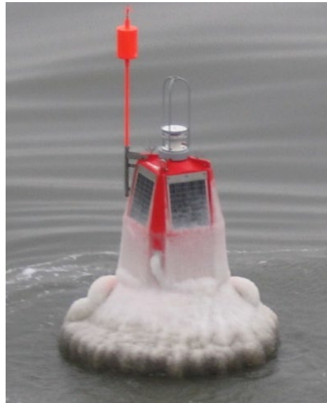
Figure 41 An example of ice build-up on a buoy.
