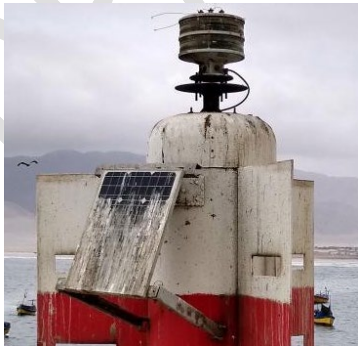
Figure 17 An example of a module affected by guano from Chile
