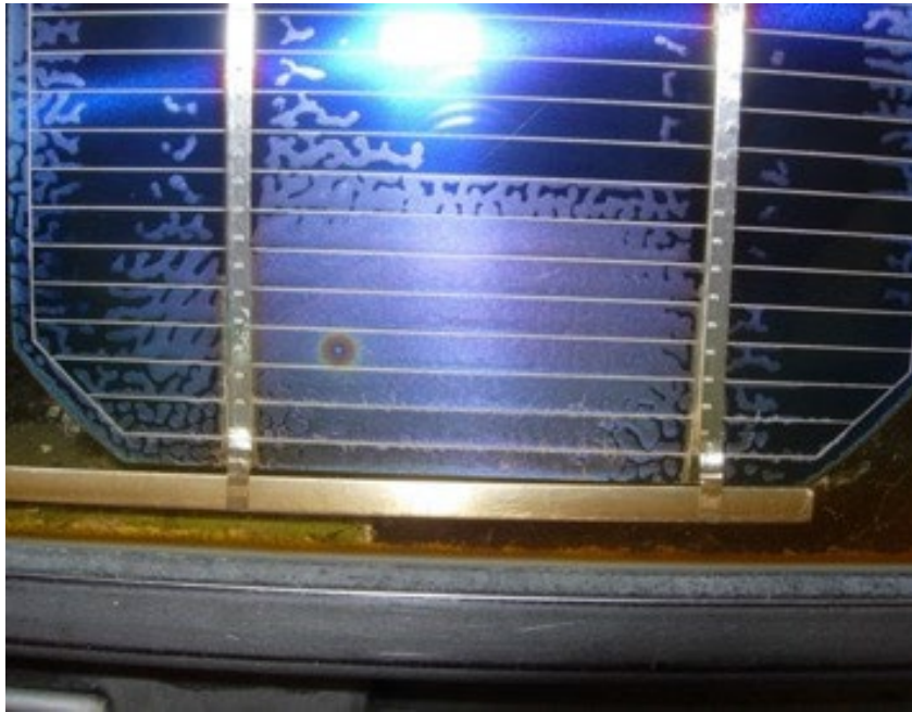
Figure 29 An example of a hot spot within a module.
