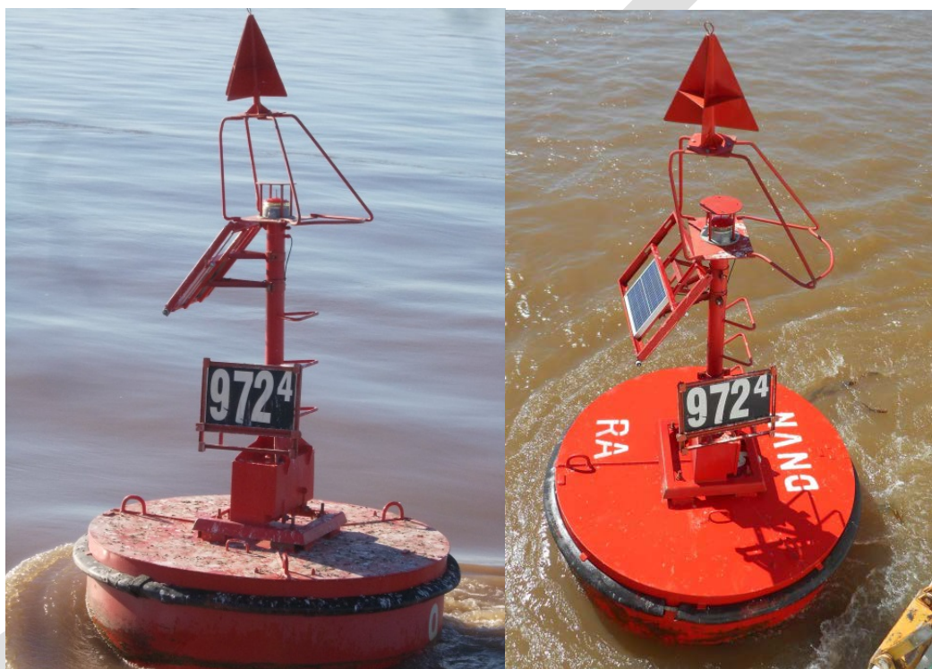
Figure 9 Buoy with modified paint system
