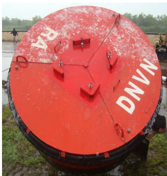
Figure 10 Buoy with additional coating applied
