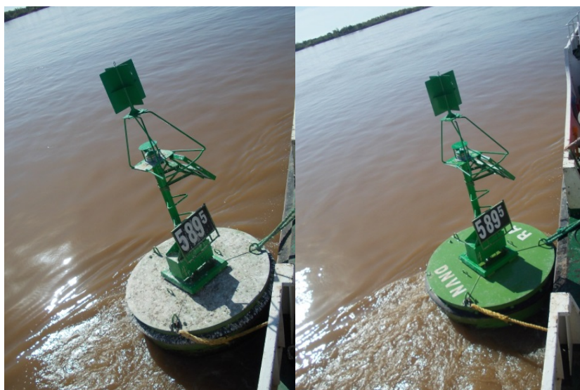
Figure 11 Coated buoy before and after pressure washing
