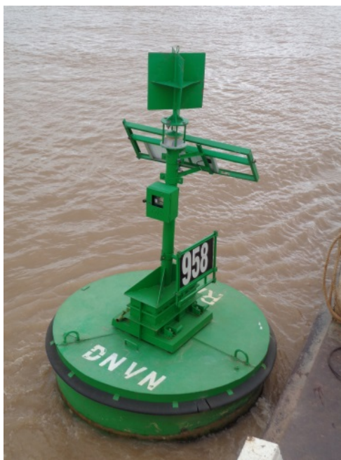
Figure 5 Buoy with audible bird scarer
