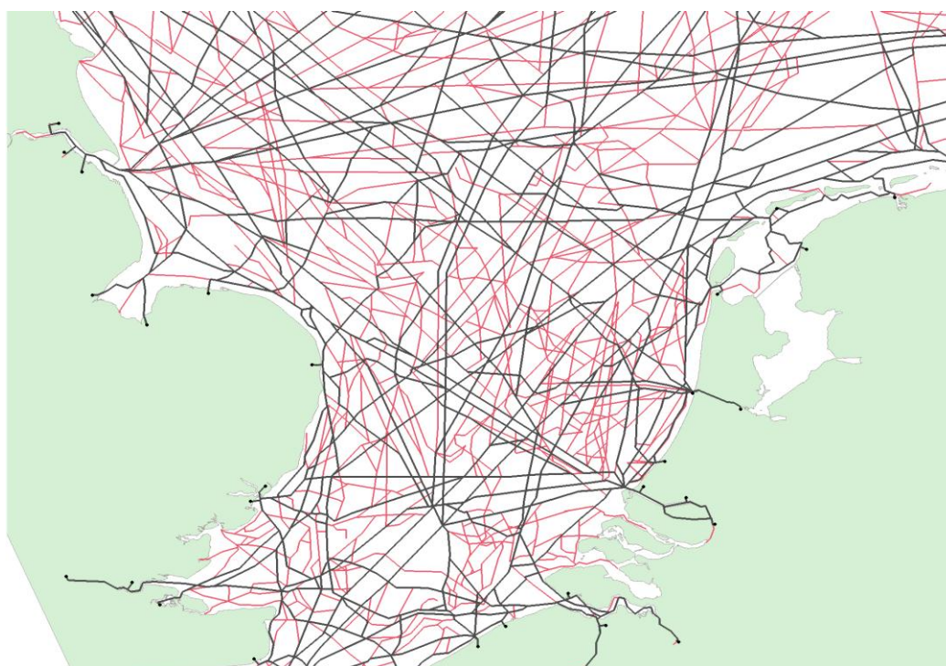
Figure 33: Applying a 'shortest path' analysis port-to-port to Figure 32 for the southern entry to the NSR (highlighted in black)
