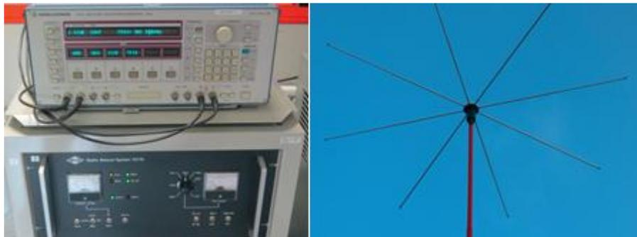
**Figure 22 - MF Transmitter (left) and MF antenna (right) used in the test.**
