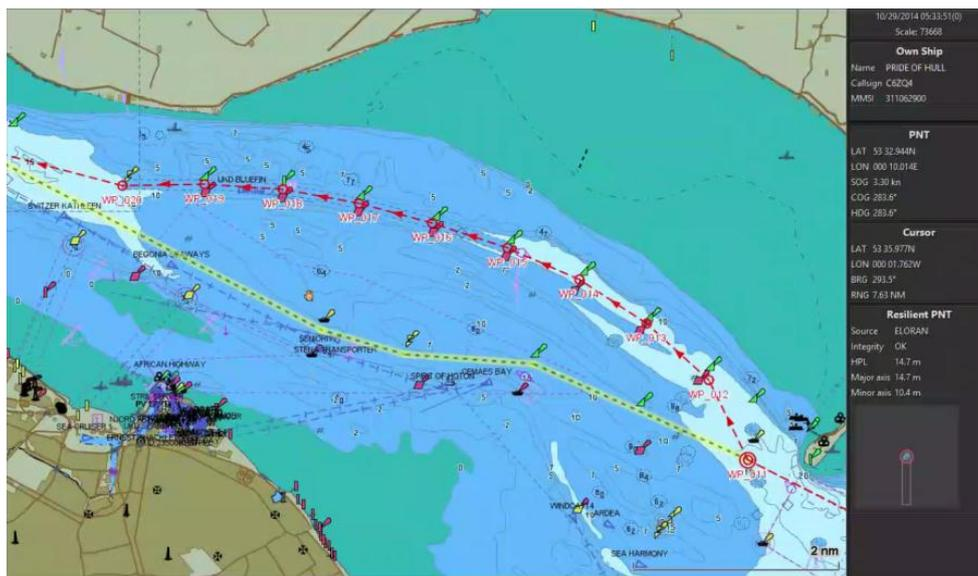
Figure 15 - EPD display panel showing PNT and Resilient PNT information on the data panel on the Right Hand Side.
