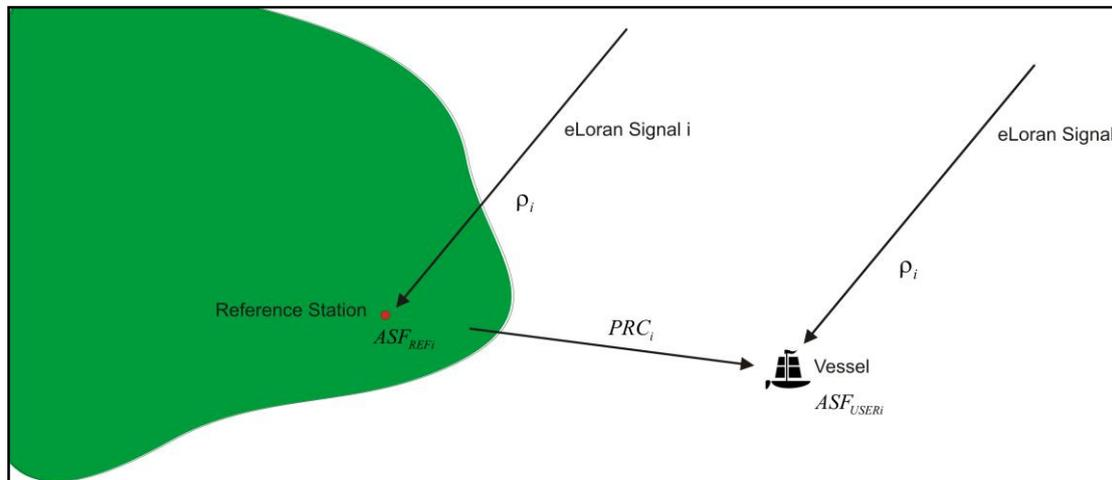
**Figure A.5 – Principle of operation of differential-Loran.**
