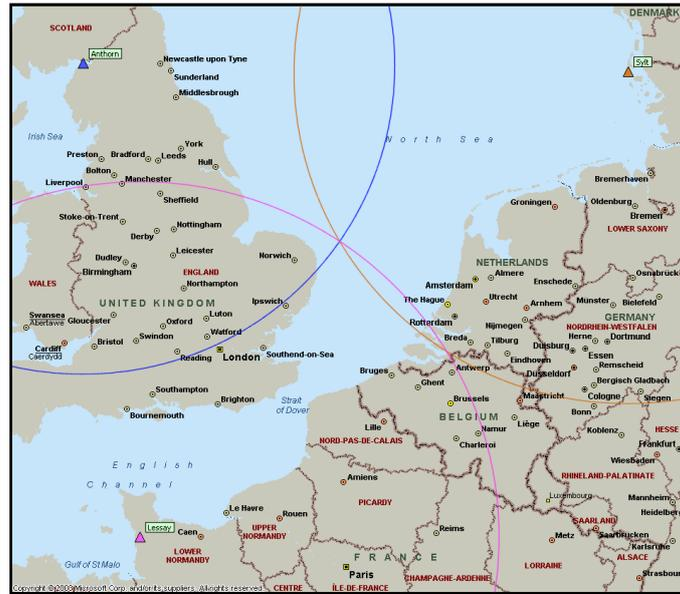
**Figure A.1 - Example of circular positioning using Anthon, Lessay and Sylt.**
