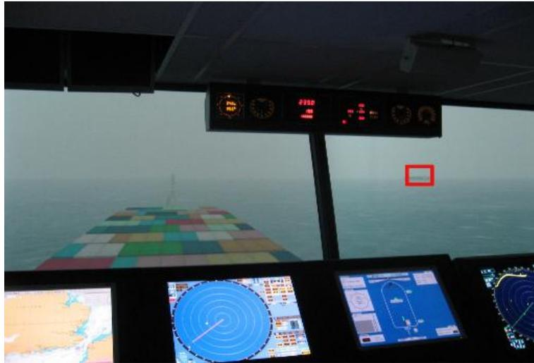
**Figure 3 - Indication of dangerous target projected as a red box on the bridge window.**
